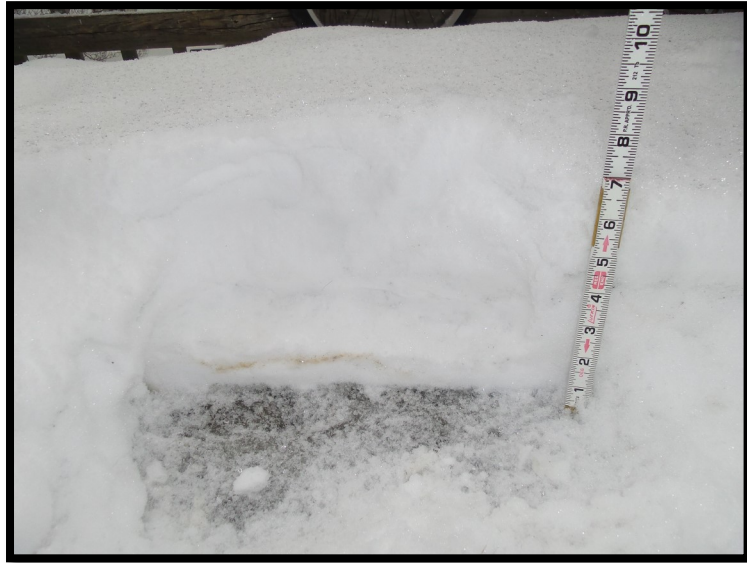
Track sectioned down the middle to show the compression of the snow under the track. The stick rule is used to measure depth of the track as well as depth to the ground if possible.
