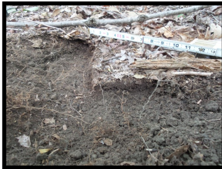
Make a crosswise cut across the width of the track in the middle.
